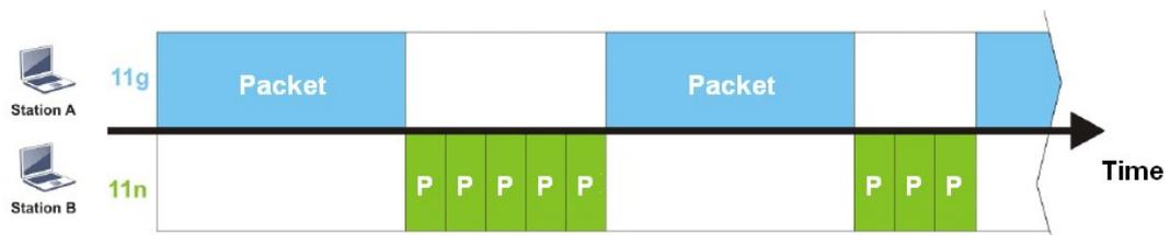
It is similar to the automatic Bandwidth Limit. The dynamic bandwidth limit of each station depends on the instant active station number and airtime assignment. Please note that Airtime Fairness of 2.4GHz and 5GHz are independent. But stations of different SSIDs function together because they all use the same wireless channel. IN SPECIFIC ENVIRONMENTS, this function can reduce the bad influence of slow wireless devices and improve the overall wireless performance.
