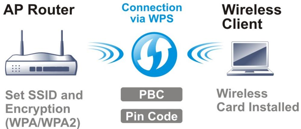
It is the simplest way to build connection between wireless network clients and VigorAP 805. Users do not need to select any encryption mode and type any long encryption passphrase to setup a wireless client every time. He/she only needs to press a button on wireless client, and WPS will connect for client and VigorAP 805 automatically.
